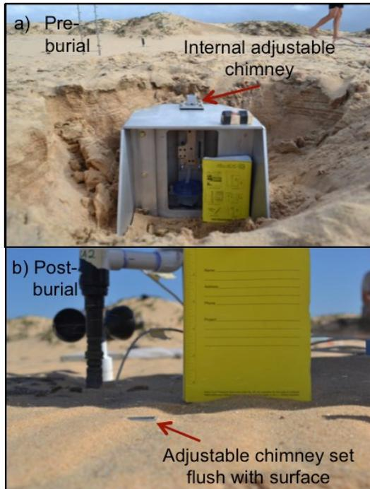
*Figure 2: Diagram showing the deployment of the Swann and Sherman (2013) bedload trap: a) pre-burial showing the outer housing case, internal adjustable chimney and bedload collection vessel, and b) post-burial of trap showing the adjustable chimney aperture set flush with the surface.*
