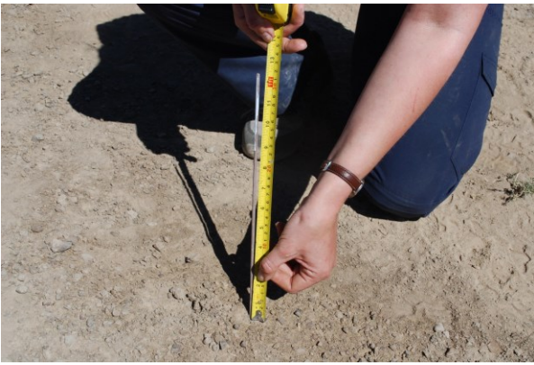
Figure 4: Measurement of distance from ground surface to top of pin.
