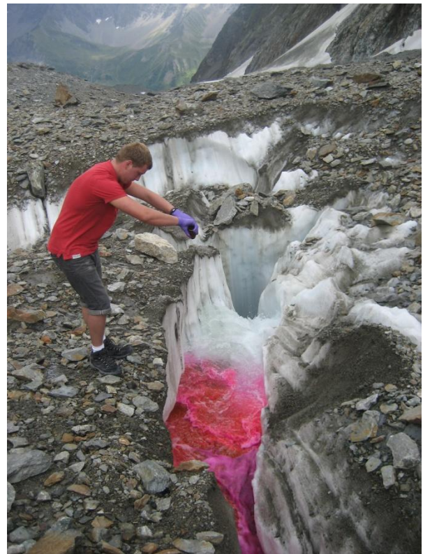
Figure 2: Injecting rhodamine WT liquid dye into a moulin on Miage Glacier, Italian Alps.
