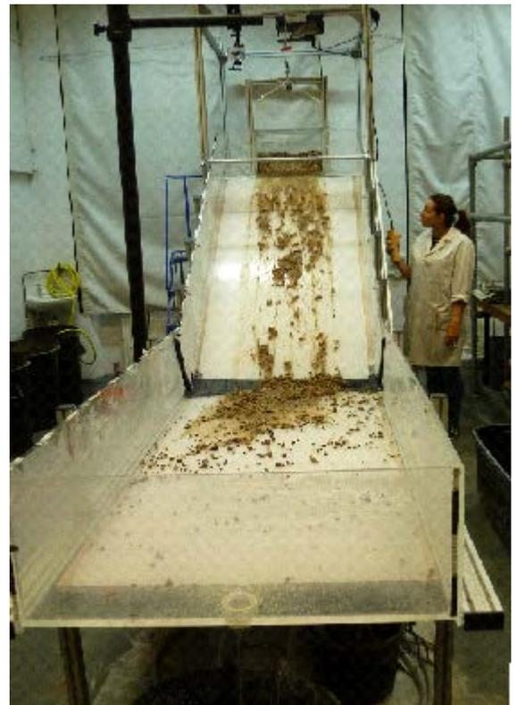
**Figure 1.** Lahar simulation flume, set at 35 degrees. The feeder box is operated remotely using an electronic winch.
